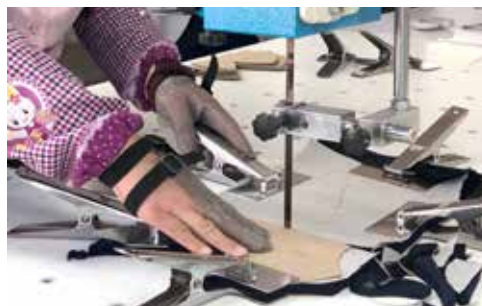
A safety measure for working with band knife cutting machines at the factory of a contract manufacturer in China
